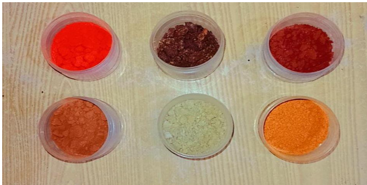
Dyes formed after diazo coupling reactions of various aromatic amines with \alpha / \beta naphthols.
